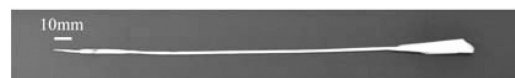
Fig. 1 Sparkling fireworks before ignition. (Black powder is wrapped in paper at the left end.)
