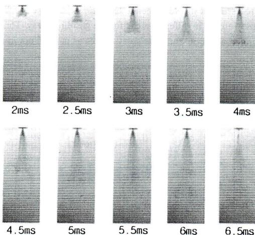
Fig. 3 Spray images by shadowgraphy ( $P_i=0.3\text{MPa}$ )
