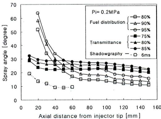
Fig. 7 Spray angles by different measuring method
