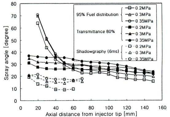
Fig. 8 Injection pressure effect
