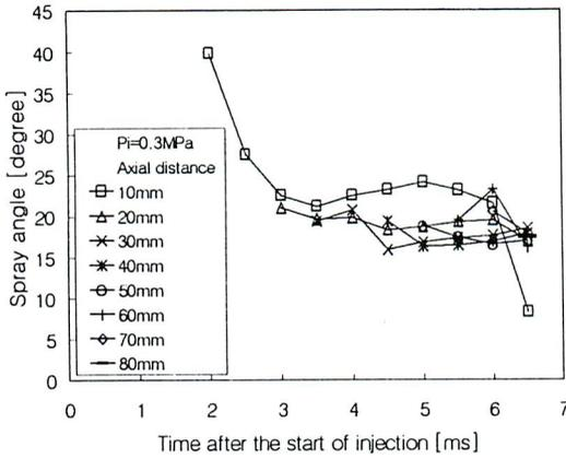
Fig. 5 Spray angle variation with time after injection by shadowgraphy
