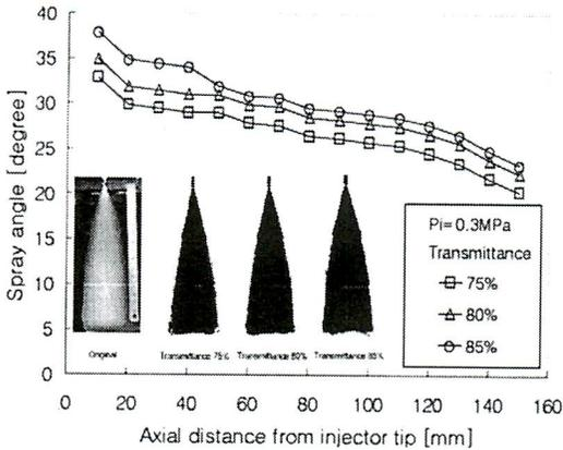
Fig. 2 Transmittance effect
