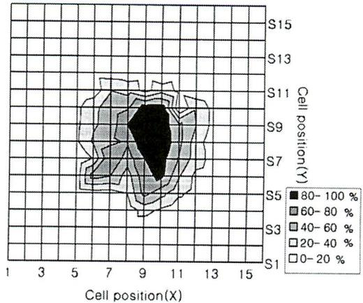
Fig. 4 Spray volume distribution in patternator
