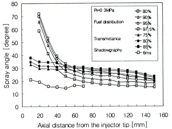
Fig. 6 Comparison of spray angles by measuring techniques
