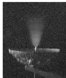
Fig.6 Electrostatic spray of YSZ colloidal solution in Mode III.
